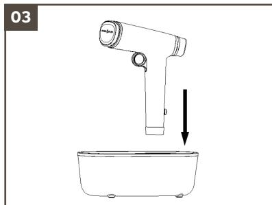
+ After warm-up, the blue indicator light is solidly on, at this time, you can remove the main unit from the reservoirs base, press and hold the Steam button as indicated by the arrow and spray steam to take care of the clothes you need.
