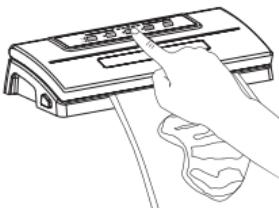
4. When SEAL indicator Light turns off, process completed. Press unlock button at both ends to open the lid and remove the sealed bag.
