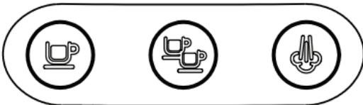
“” Power button: press power button, on display screen Single Cup → Double Cup → Steam/ Preheat will light on in turn for 1 sec. When these 3 lights flash together preheating will start. After around 1 min, 3 indicator lights will stop flashing, preheating will be finished.
