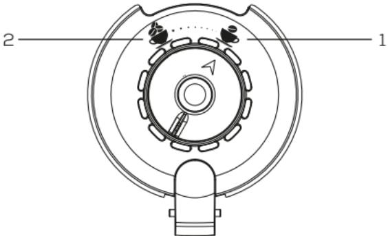
By use of the aromatisation unit on the coffee pot, you can make your coffee even more delicious. To use the aromatisation function, rotate the button from position "1" to position "2".
